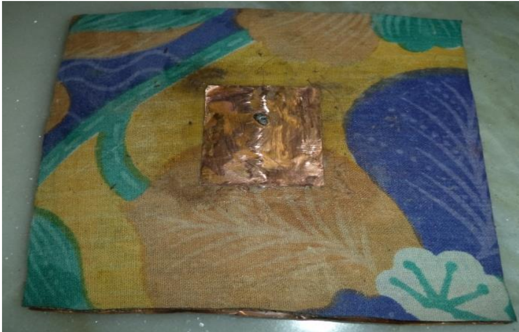
Fig 3:- Textile bed sheet cotton antenna
