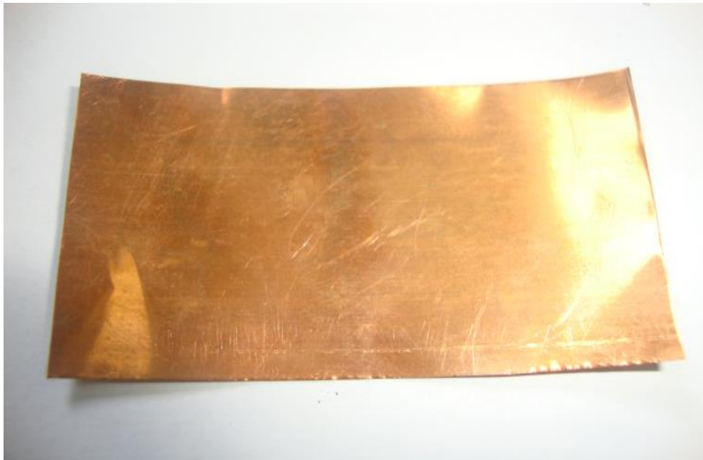
Fig: 2- Copper foil for Ground plane and Patch
